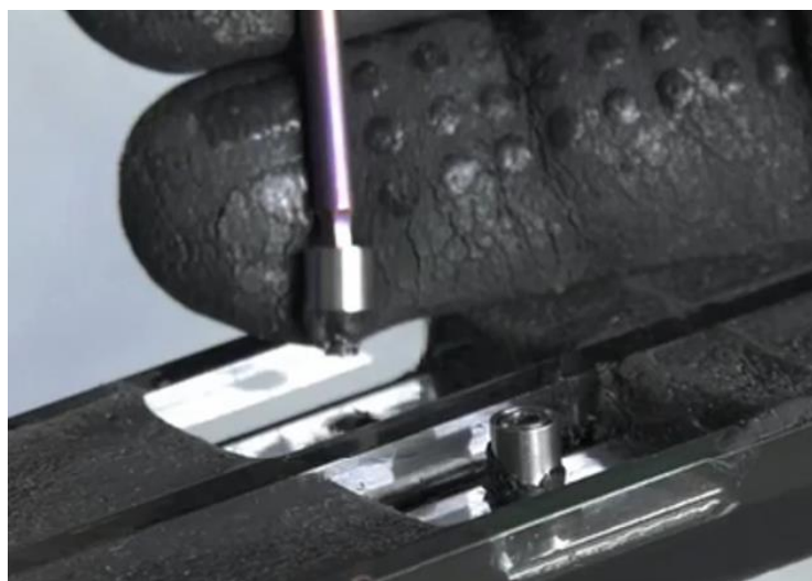
Fig. 11 SWS Air installation into insulating glass unit
