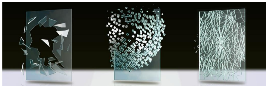
Fig. 2. Type of glass breakage (from left to right: annealed, toughened, and laminated glass panes)
