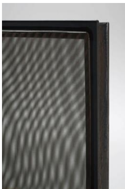
Fig. 23 Moiré effect in insulating glass unit
