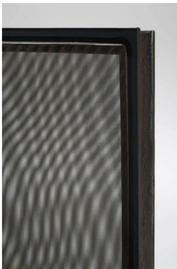
Fig. 26 Moiré effect in insulating glass unit
